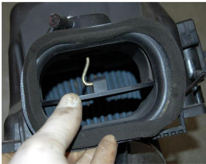
9. Remove the 4 screws that hold the butterfly in place. You can also remove the 1 screw that holds the vacuum canister in place if you would like to remove it. Also, remove all vacuum lines.
