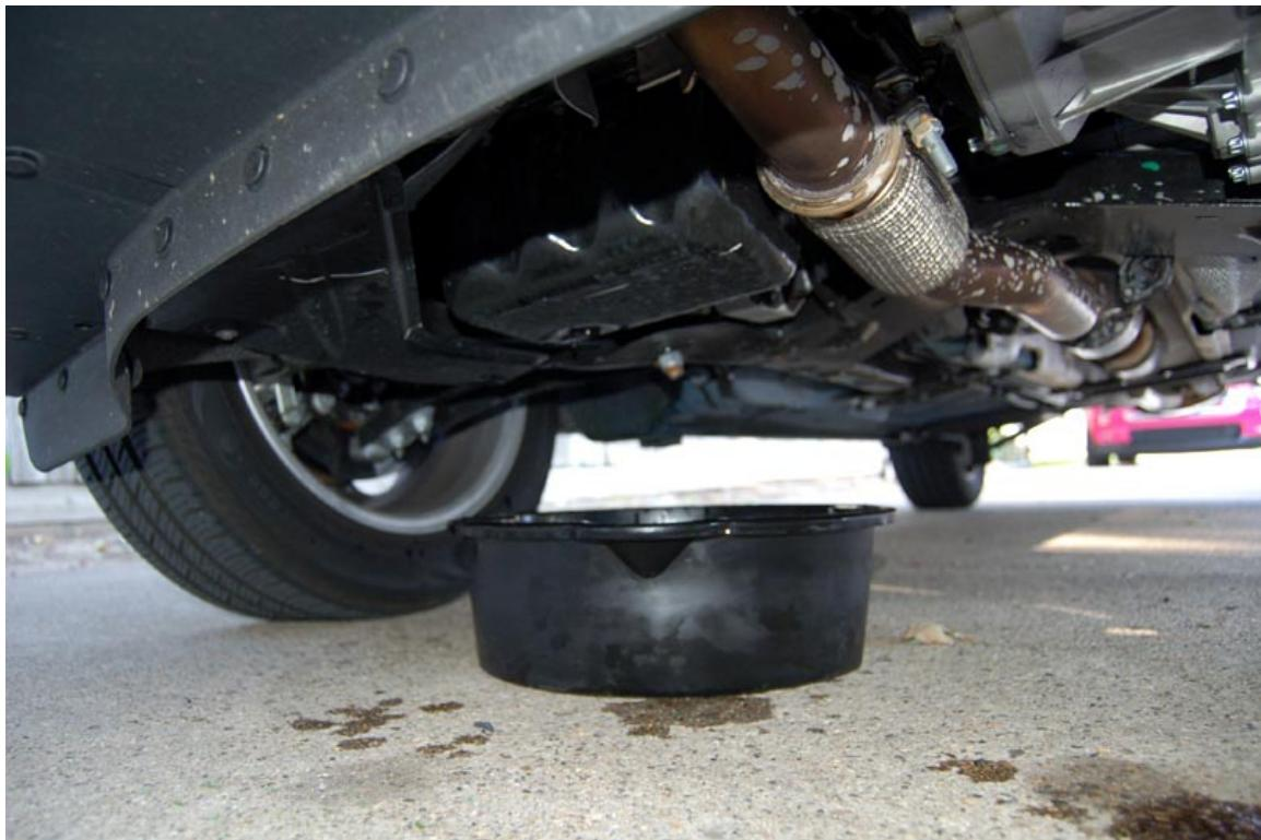
6. On the bottom of the oil pan you will find the drain plug. You will need the #8 Allen wrench to take it out.
