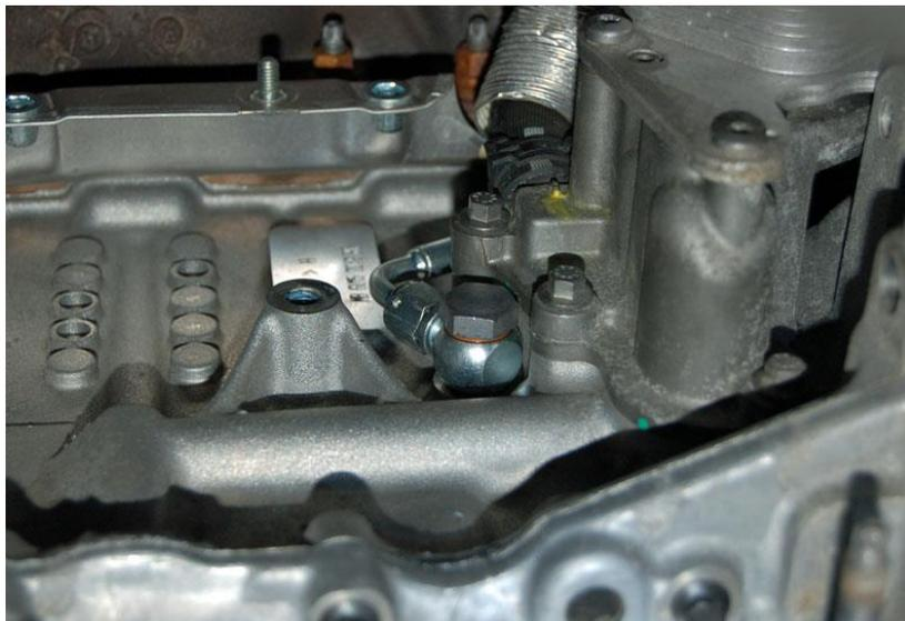
6. Install the other banjo fitting loosely onto the 90 degrees' end and then install the banjo bolt and crush washers to the cleaned area.
