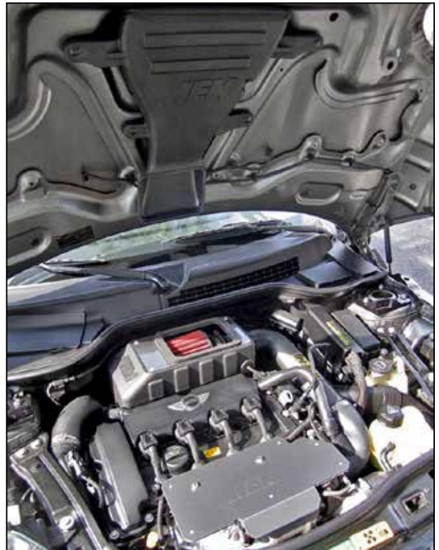
AEM® intake system installed
