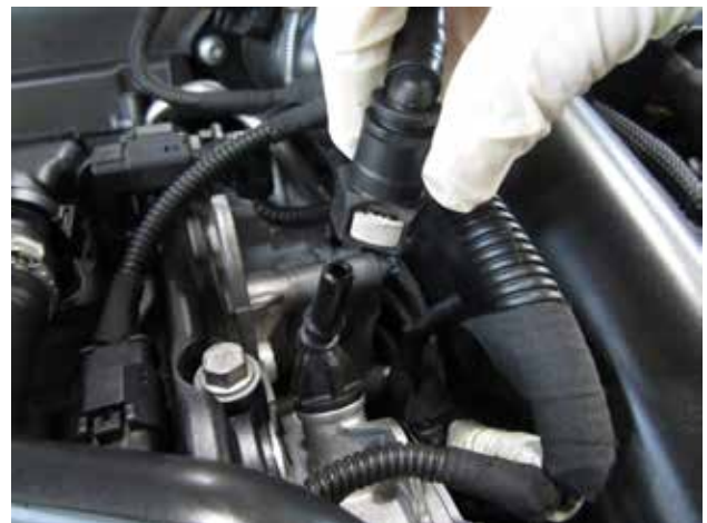
d. Disconnect the vacuum line port.
