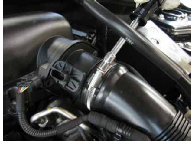
b. Loosen the hose clamp behind the MAF sensor housing.
