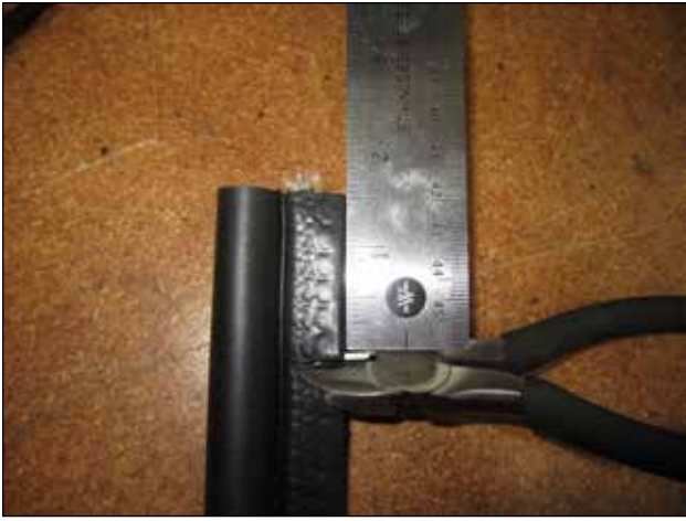
g. Cut slits in the edge trim seal on one side of the clamp using a razor or wire cutters about 1-1/2" [~38mm] from each end. Cut through the rubber clamp only. Avoid cutting the metal clips inside the clamp.
