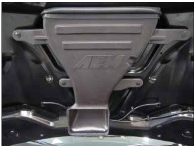
l. Mount the AEM® cold air intake scoop onto the mounting holes using the 4 plastic push rivets. Make sure the rivets are fully seated. Tuck the edge trim as needed to complete the seal around the air inlet.
