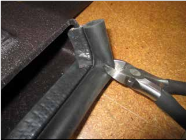
i. Cut reliefs in the 2 bent corners of the bulb seal. This will allow the bulb seal to conform to the shape of the hood.
