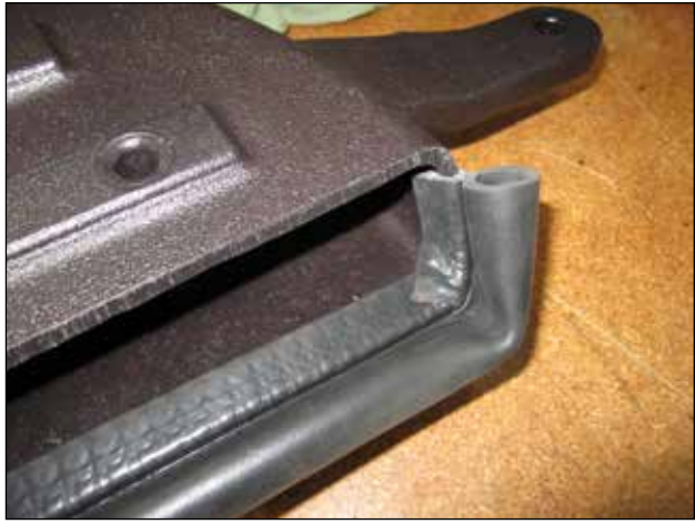
h. Install the edge trim bulb seal onto the lower edge of the AEM® cold air intake scoop. Overlap the slit ends to prevent binding around the 2 lower corners. Fully seat the trim with a rubber mallet or your hand.
