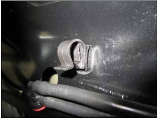
j. In most vehicles, you will need to disengage the washer fluid hose from the middle clip at the rear of the hood. Remove the clip and orient the check valve on the hose as shown.
