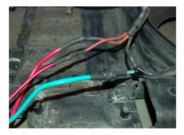
9. Once the wires are soldered and cool, slide the shrink wrap into place and apply heat gun to the area to shrink and cover the exposed wires. Work with one wire at a time and only melt one shrink at a time. If you do not have the heat shrink, use electrical tape to wrap the bare wires well.
