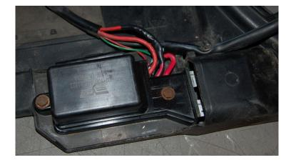
**13.** Place the cover back on and re-attach screws. Take care to make sure no wires are pinched and at attached to all stock locations like shown. Tighten screws down until tight. Do not over tighten.
