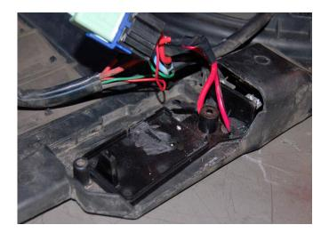
**11.** If you have a two-plug system you have a relay that needs to fit into the cover. Grind part of the case so that the relay can lay flat and hook into the top post to keep it from moving around. The final look should look like the photo in step 12.
