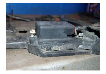
**3.** Remove both the screws and open the cover that is lightly glued over the wires. Don't worry about breaking this cover as you will not reuse any of these parts other than the two screws. If you can not get the cover off, you can just clip the wires close to the case and set it aside.
