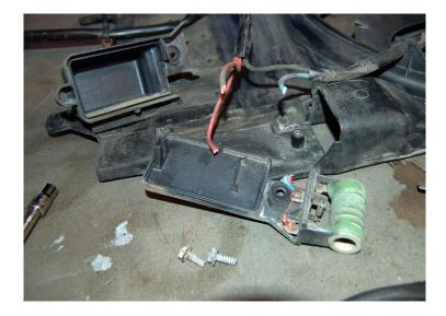
**6.** Cut the wires as close to the terminal so that you have as much wire as you need to make the install go smoothly.
