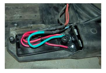
10. Tuck the wires so that it's neat and clean and that no wires are pinched or rubbing.
