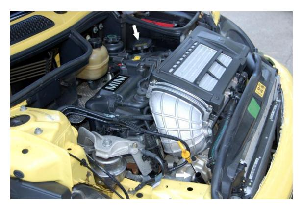
**5.** While the oil is draining, lower the car. Open the fill cap and pull up on the dipstick to let air into the system to help the oil drain. The dipstick likes to stick in its tube, so give it a small twist before you pull up on it to make sure it will pull out. Cooper dipsticks are in the front of the motor.
