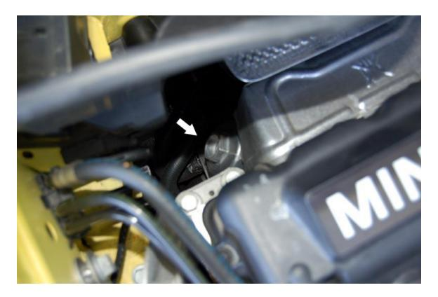
**6.** Here is where you will find the oil filter canister. If you have a strut tower brace or oil catch can in place you may have to remove it to gain access to the canister.
