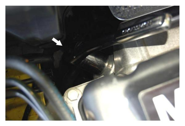
7. Use the 36mm socket to take the load off the canister and spin off till the o-ring is unseated. Do not remove it fully from the engine yet. The filter is full of oil and it is best to let it drain back into the system. It's best to let it drain for about 5 minutes so most of the oil is drained out of the filter. Once it's drained remove it.
