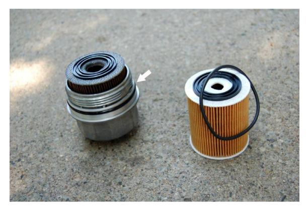
9. Remove the filter and o-ring out of the housing. For Cooper owners, make sure you do not pull out the center spring-loaded cartridge. Clean the canister and the threads/o-ring groove.
