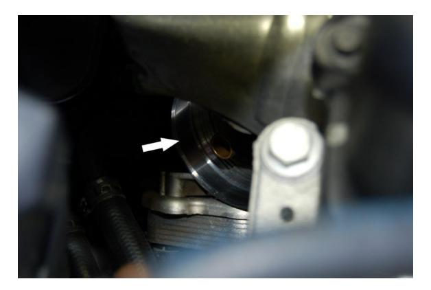
8. Here you see the housing with the filter canister removed. Take a paper towel and clean out old oil and grit to get it ready for the new filter.
