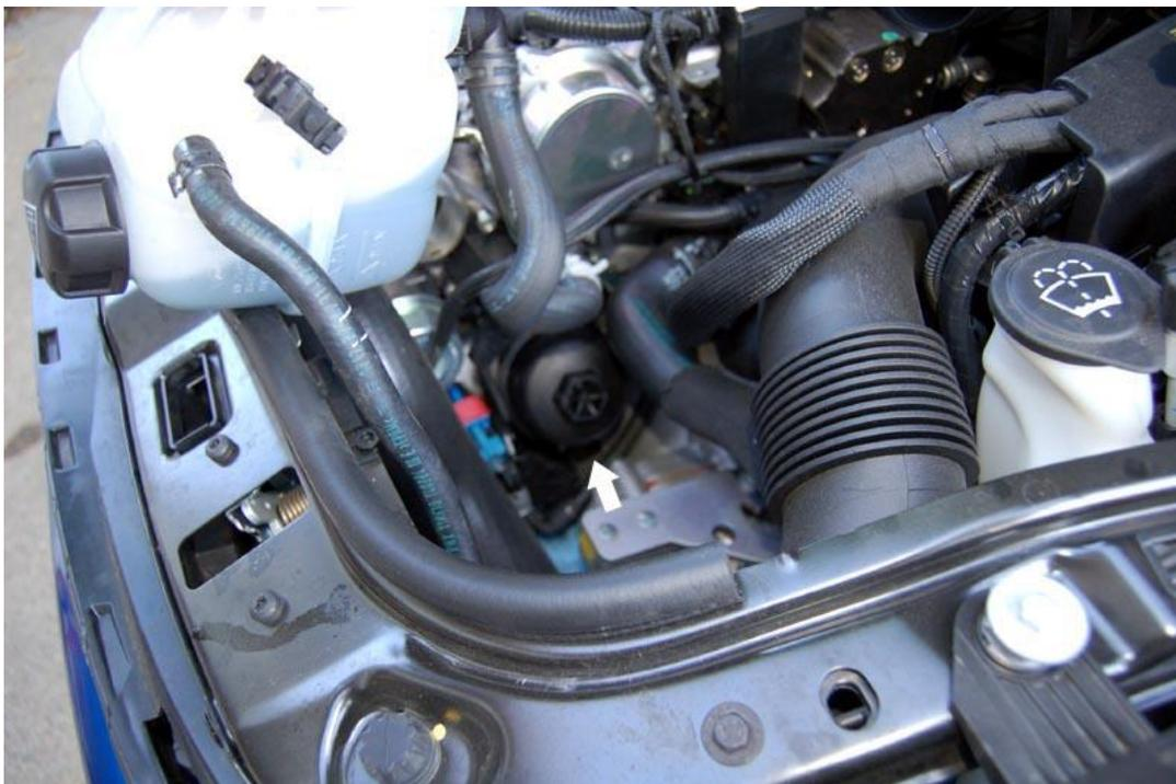
4. While the oil filter is draining, you should jack up the car to drain the pan. Remember to use jack stands whenever you or anyone else is under the car.
