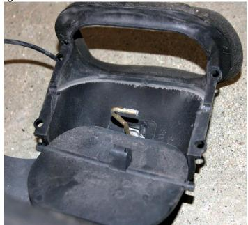
11. Cover the hole with a suitable tape of some sort. We use a heat reflective tape. Clean the area first so that the tape will stick. Cut a section big enough to cover the hole and seal it up. The only reason we are covering the hole is to keep any warm air from the engine bay from entering into the intake path. Once the intake is sealed to the hole in the firewall, it will draw air from the cowl.
