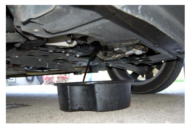
**4.** Remove drain plug with the 13mm socket and drain the oil into a drain pan.
