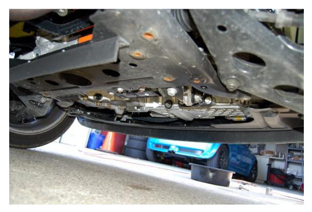
**3.** Find the drain plug under the car, on the back of the oil pan.
