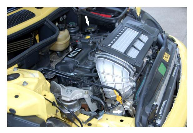
5. While the oil is draining, lower the car. Open the fill cap and pull up on the dipstick to let air into the system to help the oil drain. The dipstick likes to stick in its tube, so give it a small twist before you pull up on it to make sure it will pull out. Cooper dipsticks are in the front of the motor.
