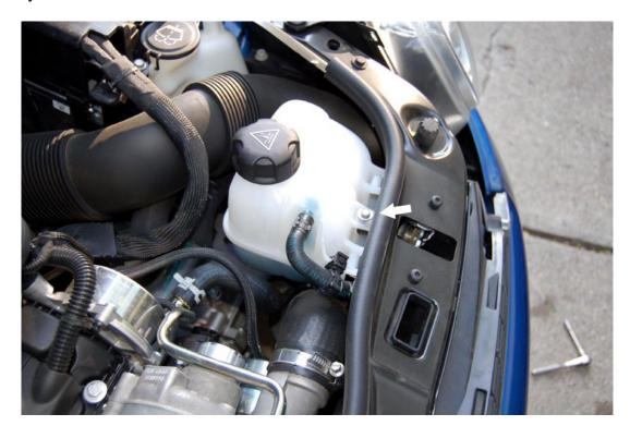
3. You can then swing the bottom of the tank out and then pull up, and it will come off the posts that it is sitting on. Lean the tank towards the center of the car without disconnecting anything. You can now see the oil canister. Use the ½" drive and extension w/ 27mm socket to take the load off the canister and spin off till the o-ring is unseated. Do not remove it fully from the engine yet. The filter is full of oil and it's best to let it drain back into the system.
