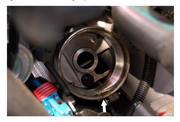
**9.** Properly dispose of the oil filter and remove the o-ring from the canister. Clean up the canister, add the new o-ring and the filter. Be sure to pre lube to o-ring with fresh oil before you put the canister back in the housing. Start it by hand to make sure you have proper thread engagement, and then tighten down to 25 Nm (18 ft. lbs or 221 inch. lbs.).
