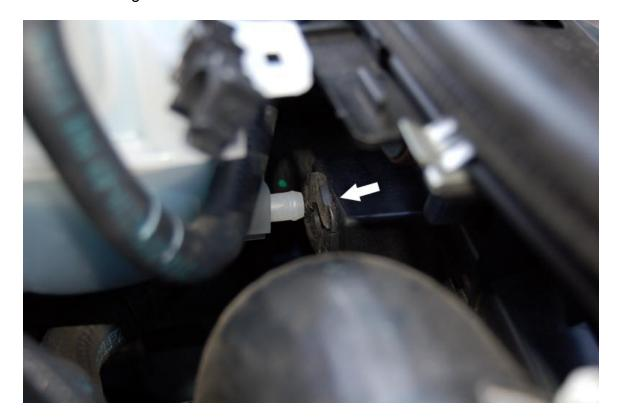
**11.** Fill the engine with 5 quarts of synthetic motor oil and replace the oil fill cap. Start the engine, let it run for a few seconds and then turn it off. This will allow the oil to fill the filter, which will allow you to check the oil level correctly.
