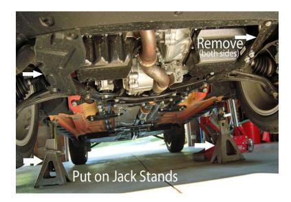
2. Remove the two support bars shown in the photos. Reinstall the two large bolts back into the crush tubes. Torque them to 7 ft. lbs. Remove the j-nuts and small bolts that hold the front ends of the support bar. Put them in a box and save them in case you ever need them.
