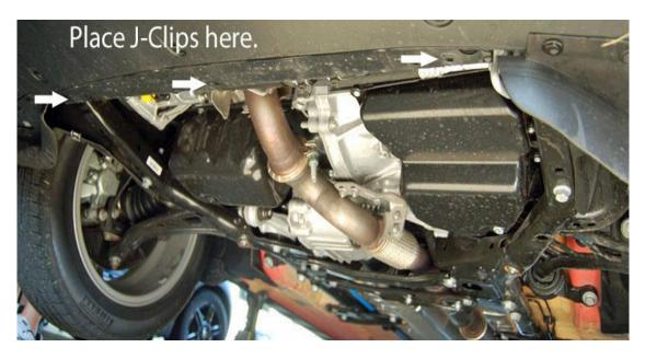
**4.** Next remove the two bolts that hold the lower sub-frame support to the sub-frame. We will use new longer bolts to attach the skid plate, but the support must be put back into place, so it will be reused. It will only go on in one direction due to the tab on one side.
