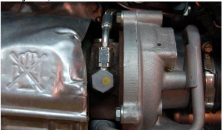
**5.** Take the line and fish it down thru the engine. Make sure the 90-deg. end is down (against the engine) as shown in the photos. Now loosely install the 15 degrees' end to the turbo banjo fitting.
