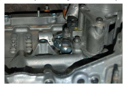
**6.** Install the other banjo fitting loosely onto the 90 degrees' end and then install the banjo bolt and crush washers to the cleaned area.
